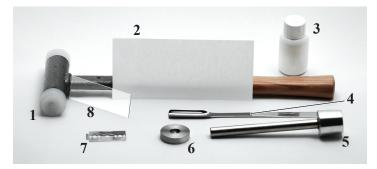
**Figure 2.** Photograph of the sample preparation components to compress powders into a pellet. 1: recoil-free hammer, 2: piece of paper, 3: powder sample, 4: spatula, 5: tappet, 6: sample holder, 7: razor blade, 8: glass/microscope slide.
