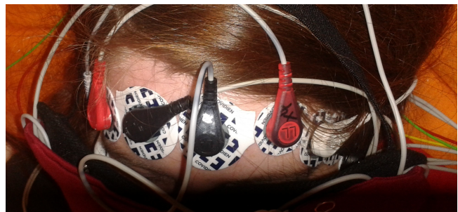
Figure 2.14: Sticky electrodes of both systems were placed on the forehead, recording EOG and frontal EEG.
