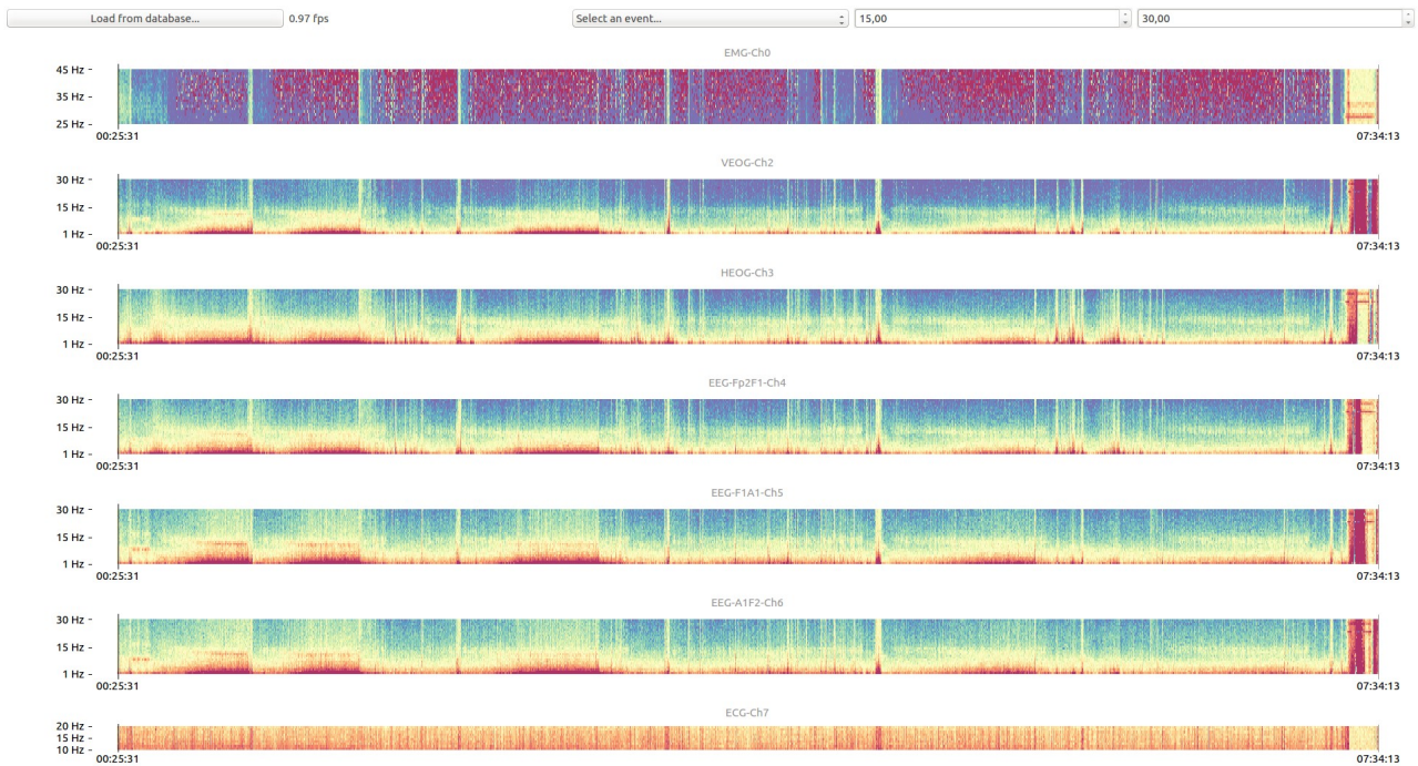
Figure 3.6: Time frequency plots of a whole night recording of the Traumschreiber system of all relevant channels (the channel between the chin and the bottom eye electrode is not depicted). Note the clearly visible activity in the slow wave and the sleep spindle frequencies, and the arousal/movement artifacts, which give the sleep researcher an instantaneous overview of the night.
