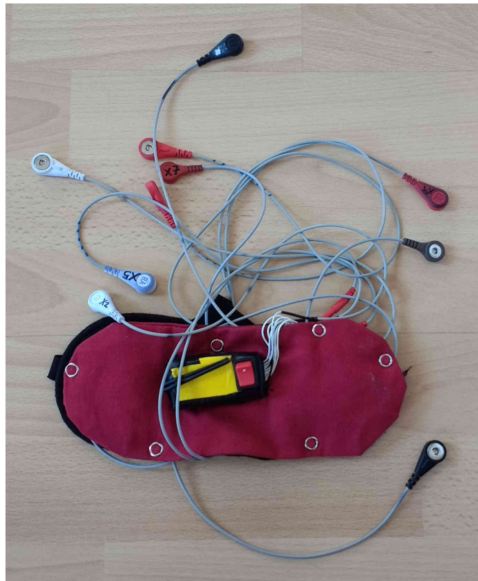
Figure 2.11: Traumschreiber sleep mask version 2.2. Note that the cables are far too long (making the sleep mask heavy and uncomfortable) and that the electronics are not hidden inside the mask.
