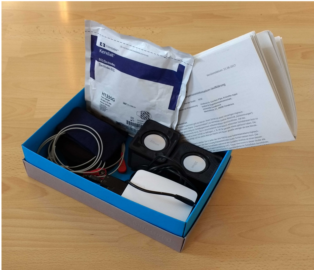
Figure 3.2: One complete Traumschreiber system experiment box, including the sleep mask, the Raspberry Pi minicomputer, the speakers, electrodes and questionnaires. Each subject receives one box, records polysomnographic sleep data at home following the instructions of the Traumschreiber system, and returns the box including the data to the experimenter. No experimenter is needed at the place of recording.
