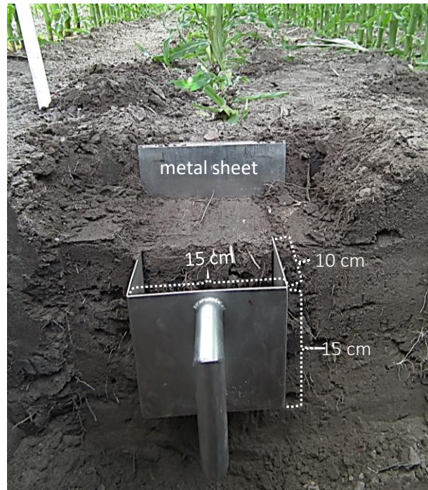
Figure 2: Usage of the soil shovel to obtain the soil-monolith sample around the banded slurry (SM 2); metal sheet = used to limit the SM in front.
