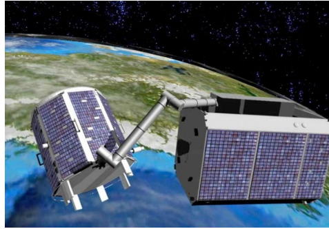
FIGURE 1.2: DEOS: German on-orbit satellite servicing robotic mission for rendezvous, capture and docking of client satellite. After the servicer (right) approaches the client (left), a robot arm mounted on the servicer grasps the client and performs the desired operations.
