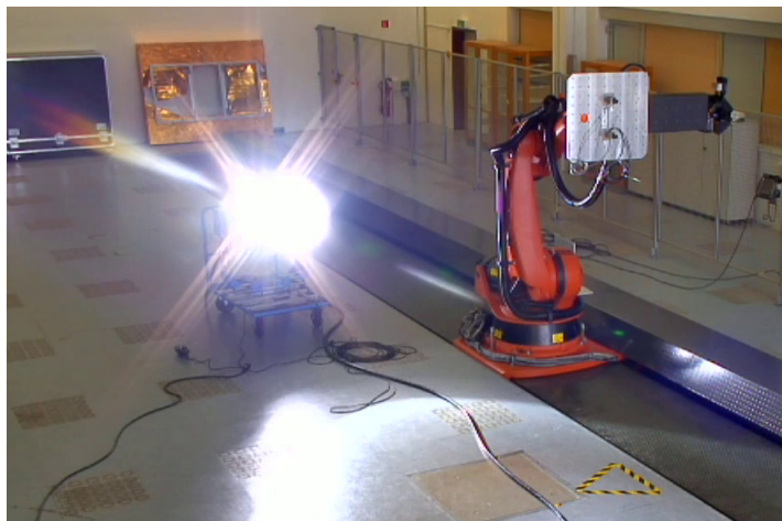
FIGURE 4.3: High-power floodlight simulates the sun at the EPOS facility.
