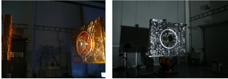
FIGURE 4.1: Satellite mock-ups reproducing full scale satellite used in various chapters of this thesis: DLR satellite mock-up with golden foil (left) in Chapter 5 and the Kayser-Threde mock-up with real MLI (right) in Chapter 6 at the EPOS facility.
