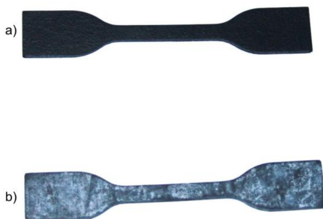
Figure 3.20 Picture with different the surface of cured samples in storage at ambient temperature for: a) A4b and b) A4e
