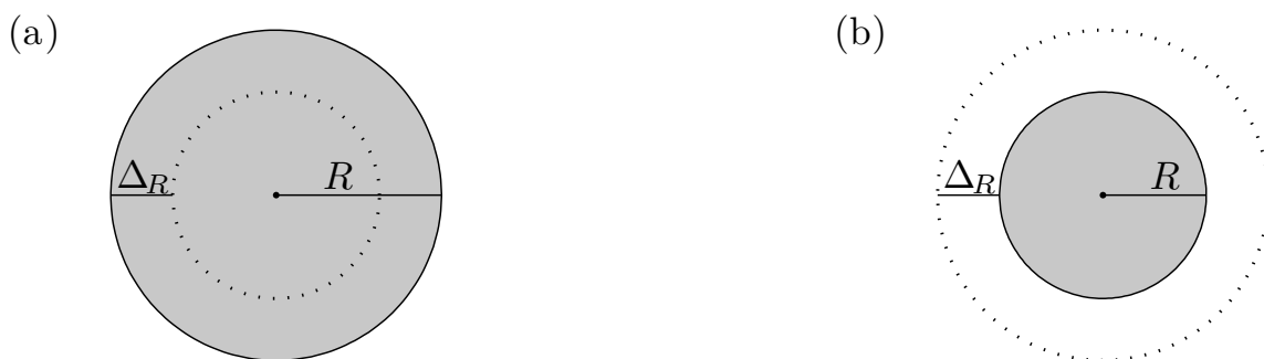
Figure 3.1: Sketch of a circular object’s geometry with its radius R in (a) the RTD and (b) the ITD setup. In both cases the dot marks the probing site and the shaded area is the so-called detection area, defined by those object center positions that turn the signal “on”. The dotted line marks the initial probability distribution displaced by \Delta_R from the absorbing boundary, see text, which is used for Eqs. (3.9) and (3.13).
