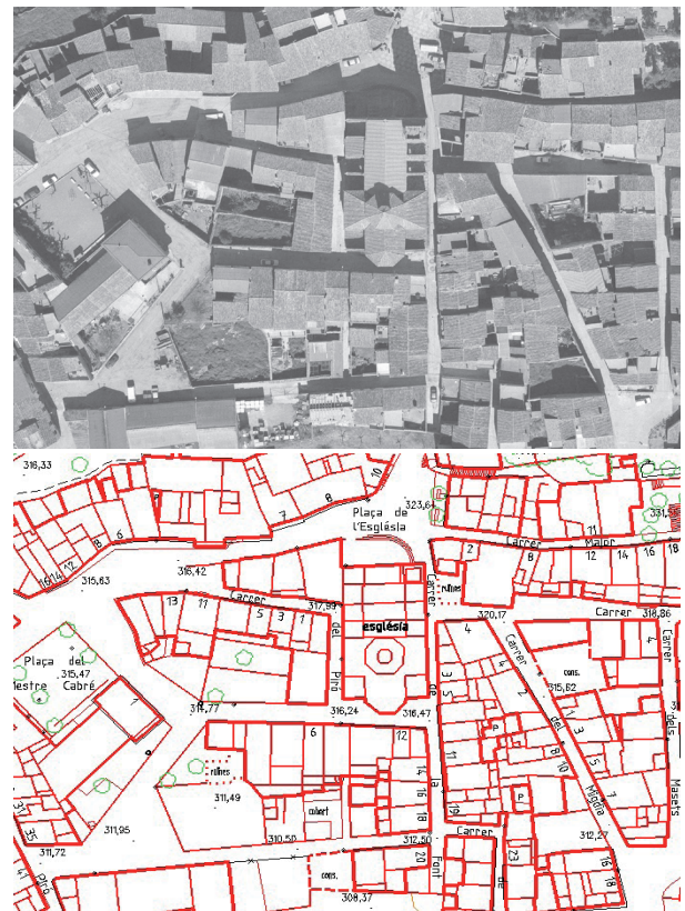
Figure 6a and 6b. Vector data generated by image stereo-mapping
