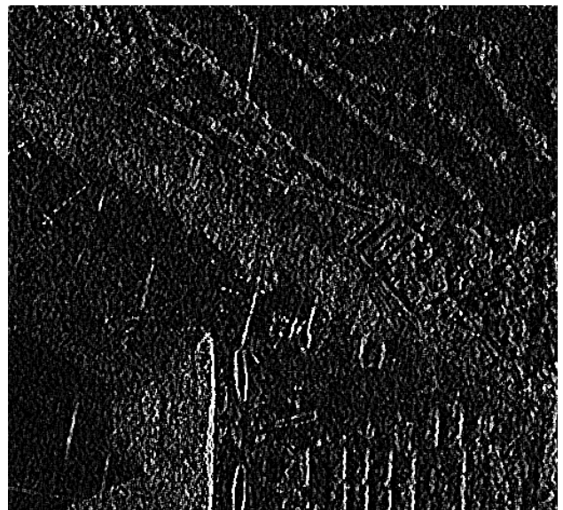
Figure 9: High pass filtered TerraSAR-X image after an inverse FFT
