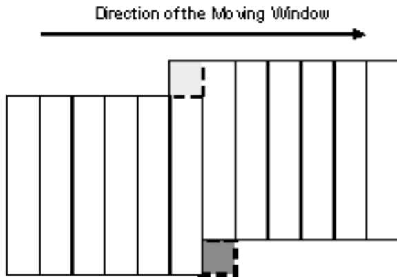
Figure 2. After the landscape metric of the first row of a map has been calculated in the following rows only single cells has to be added or subtracted from the previous calculation.
