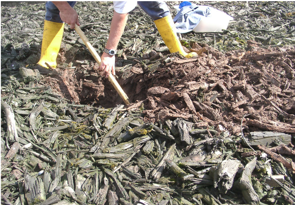
Figure 1. Photograph showing the coarse packing material in the Hamm full-scale industrial biofilter.
