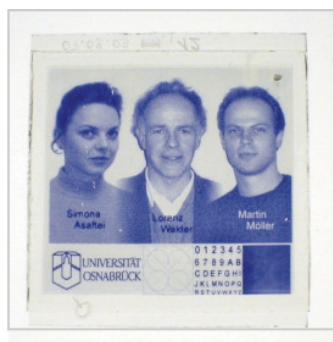
Figure 3.42. Closed electrochromic cell (CeO 2 , counter electrode, 1 M LiClO 4 ,/ethylen glycol)
