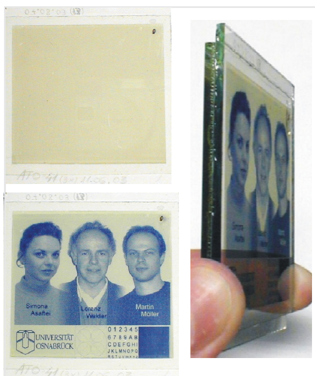
Figure 4.4. Closed cell with E-33 on the ATO counter electrode and \text{LiN}(\text{SO}_2\text{CF}_3)_2 /glutaronitrile
