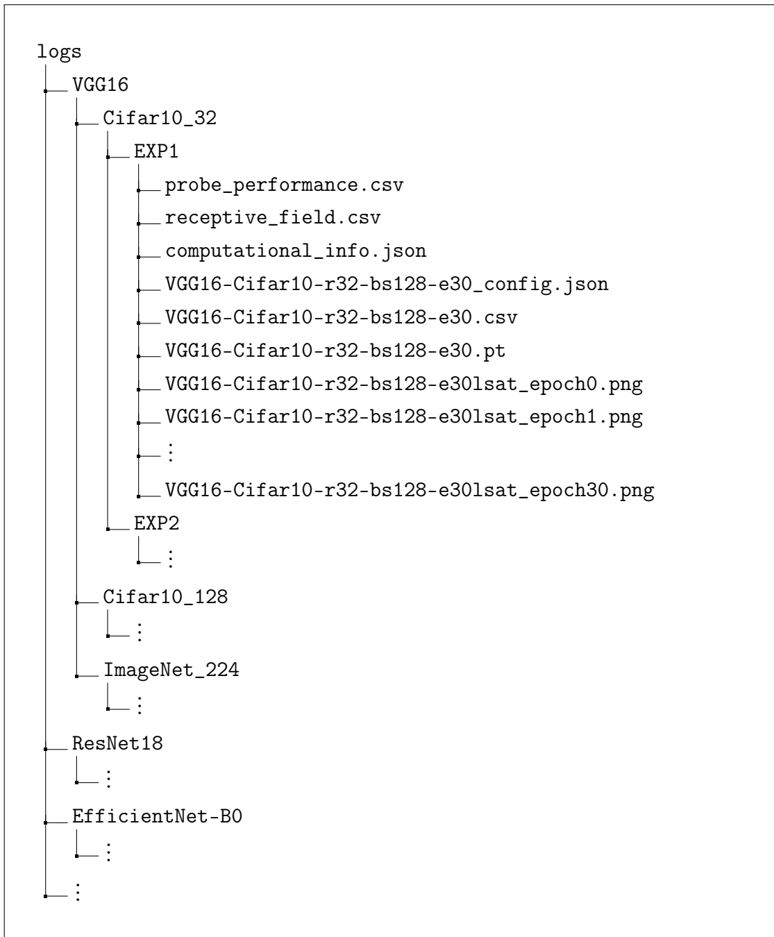
Figure 42: An example for the automatically generated folder structure used for saving experiment results in PHD-Lab. The logging structure is nested and the naming of files copied regularly are named based on the configuration to avoid confusion of experimental results.
