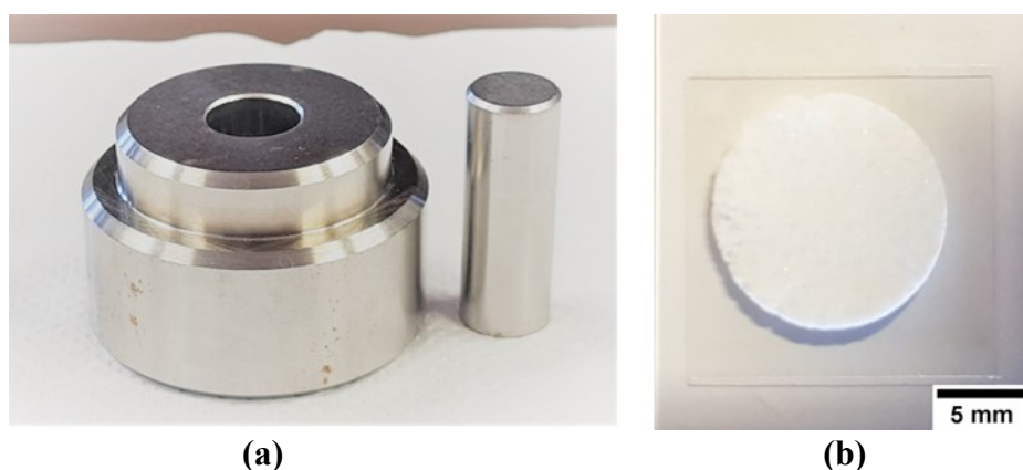
Figure 3-8 Fabrication of zinc oxide tetrapod (T-ZnO) pellets. (a) The stainless-steel pressing tool and (b) the resulting T-ZnO pellet with a diameter d of \approx 13 mm and a thickness t of \approx 1 mm.
