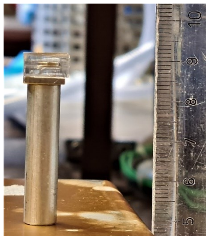
Figure 3-11 Photograph of stamp holder made of aluminum, having a PDMS layer with a permanent external magnet (NdFeB, 6 \times 1 \text{ mm}^2 (diameter*height), Grade 52) embedded.
