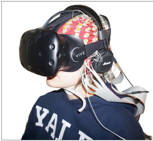
Fig. 3 Combination of VR HMD and EEG. Note. The VR equipment included the immersive HTC Vive HMD, headphones for stereoscopic sound, and the HTC Vive tracking stations for real-time head-tracking. The VR equipment was carefully arranged atop the 128-electrode EEG
