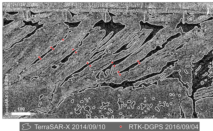
Fig. 5.3-7 Trough extraction ( white lines ) derived from TerraSAR-X data and water edges recorded with RTK-DGPS 6 days before image acquisition ( red dots )
