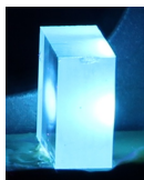
Figure 2.22 – Luminescence of an Mg-doped congruent LN crystal ( c_{\text{Mg}} = 6.5 mol%) induced by intense ultrashort fs-laser pulses with a central wavelength of 400 nm. The crystal is cooled down to 10 K in a closed-cycle cryostat.
