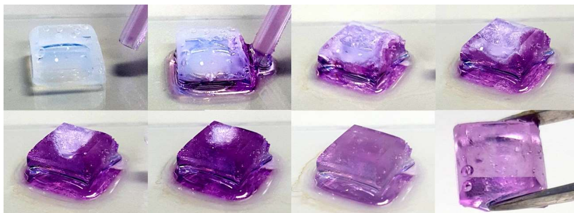
Figure 40. Photographs of the imbibition process of a silica stamp with ink (in this case a solution of C_{60} in toluene). The stamp is located on a glass slide with the structured stamp side facing upwards. The dried silica stamp is opaque and colorless. The infiltration occurs from the backside of the stamp by dropping the stamp solution onto the glass slide. The fully infiltrated stamp appears pink transparent.
