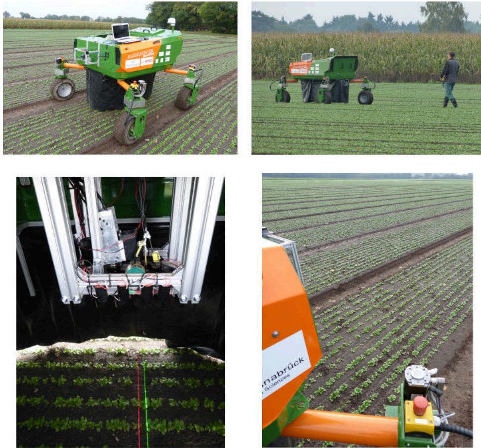
Figure 5.67: Impressions of field situation and tests of corn salad scans. Bottom/left: Sensing head of the MWLP system mounted into BoniRob with lasers turned on (NIR not visible).
