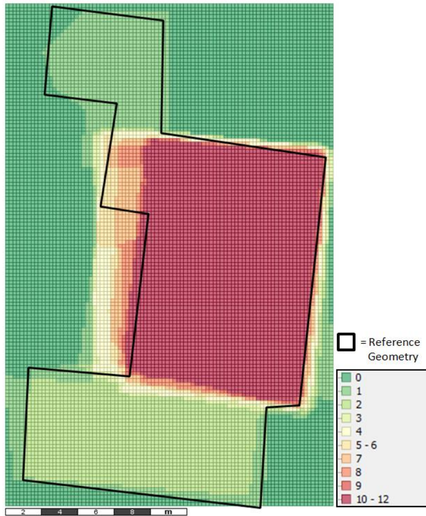
Figure 29. Number of overlapping geometries on an 18.0 m x 27.6 m raster with a cell size of 0.2 m for the building with the lowest overall quality (53.56%). (Hillen & Höfle 2015)
