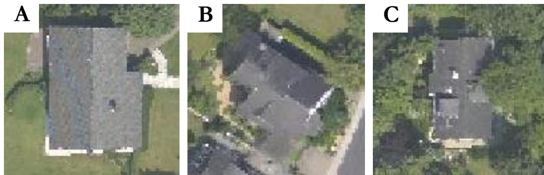
Figure 13. Three categories of building shapes. A: simple, mostly straight lines; B: complex, many edges, hard to distinguish from surrounding; C: complex, covered by trees.
