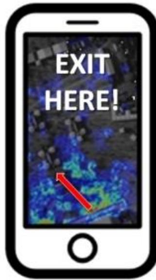
Figure 7. Schematic representation of an emergency smartphone app. The crowd density is visualized in the background. The fastest escape route is emphasized with a red arrow. (Hillen et al. 2015)
