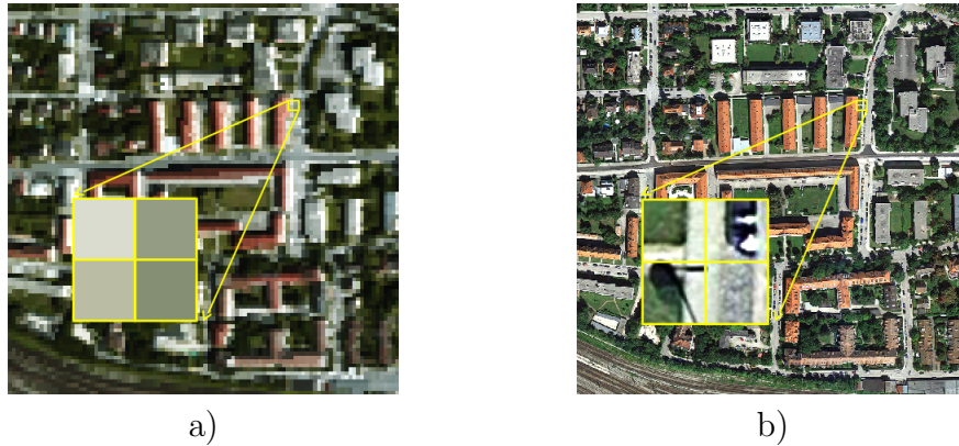
Figure 4.11: Illustration of spatial correlation among neighboring hyperspectral pixels. Pixels in the HyMap hyperspectral image (a) with a ground pixel size of 4 m are very often mixed. The mixture is usually spatially correlated, i.e., neighboring pixels contain common endmembers. E.g. all four neighboring pixels in (a) contain spectra from the road as seen in the high resolution ©Google Earth Image (b).
