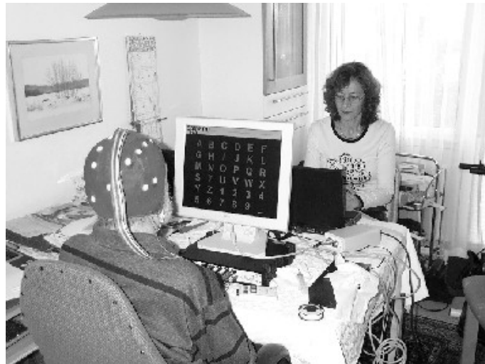
Figure 3.3: Communication facilitated by EEG-based BCI technology. The patient composes words and sentences based on voluntarily produced brain-activation patterns read of by the computer (from http://www.mp.uni-tuebingen.de/mp/index.php?id=137 ).
