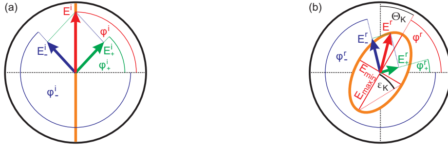
Figure 2.16: (a) Linear polarization of the incident light (superscript i ). (b) Elliptic and rotated polarization of the reflected light (superscript r ). The polarizations E^{i/r} with the polarization angle \varphi^{i/r} are described by superposition of right and left circular polarized light waves ( E_-^{i/r} and E_+^{i/r} with phase \varphi_-^{i/r} and \varphi_+^{i/r} , respectively). Furthermore, the Kerr angle \Theta_K and the Kerr ellipticity \epsilon_K as well as the minor axis E_{min} and the major axis E_{max} of the ellipse are marked.
