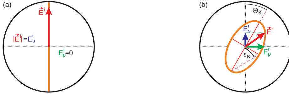
Figure 2.17: (a) Linear polarization of the incident light (superscript i ). (b) Elliptic and rotated polarization of the reflected light (superscript r ). The polarizations E^{i/r} are described by superposition of s- and p-polarized light waves ( E_s^{i/r} and E_p^{i/r} , respectively). Furthermore, the Kerr angle \Theta_K and the Kerr ellipticity \epsilon_K are marked.
