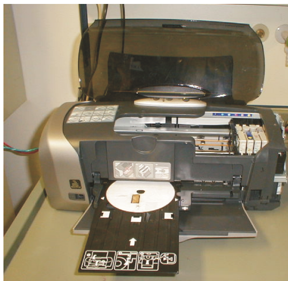
Figure 2.2 Syringe of 2 mL replaces the original ink reservoir (a). Construction for the chemical printing job (b).
