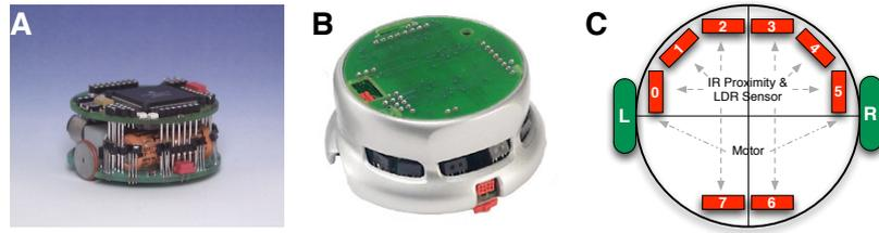
**Figure 5.1:** KHEPERA ROBOT. A) Khepera I Robot (front), B) Khepera II Robot (front), robot pictures taken from (K-Team, 2005), C) Schematic view of the sensors and actuators, redrawn from (K-Team, 1999). Green: The two actuators (DC motors). Red: the eight proximity and light intensity sensors. The indices of the sensors correspond the hardware specifications.
