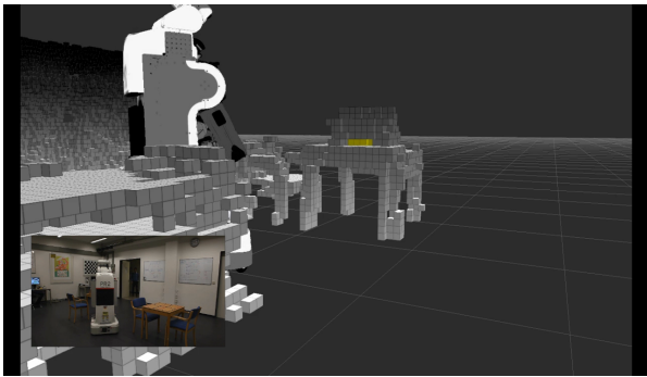
(c) When the robot reaches the other side of the table, only a few unobserved voxels inside the cavity remain unobserved.
