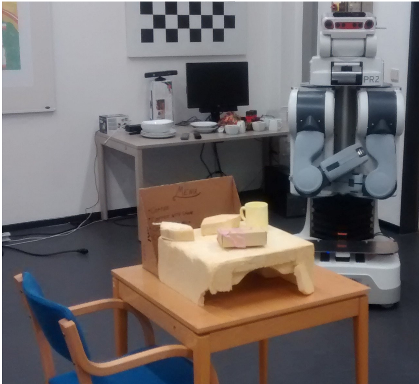
Figure 5.2: PR2 during a search process. The target volume on top of the table has several occlusions and a cavity. Figure reproduced from Gedicke et al. (2016).
