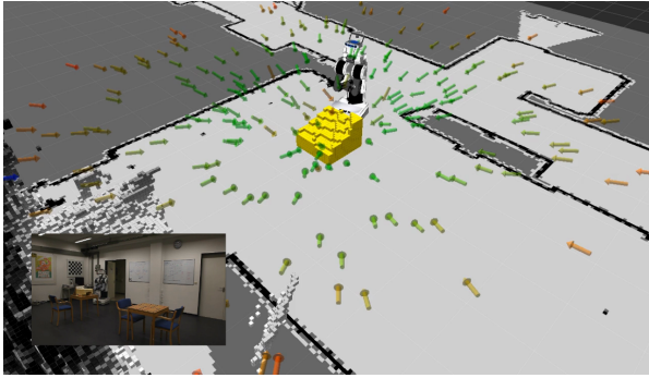
(a) Initial set of views. Part of the ROI was already observed by the robot in its initial position.
